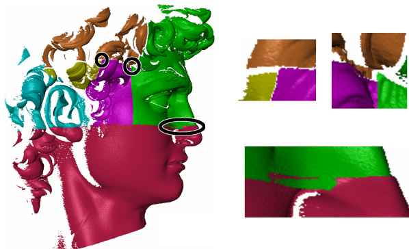
Figure 2. Hierarchical alignment [12] was used to dice a source mesh, and align the resulting pieces to a target mesh (not shown). Closeups of the circled areas show that the different pieces can overlap or drift apart substantially from each other. These discontinuities are smoothed out by the thin-plate spline computed by our algorithm.
