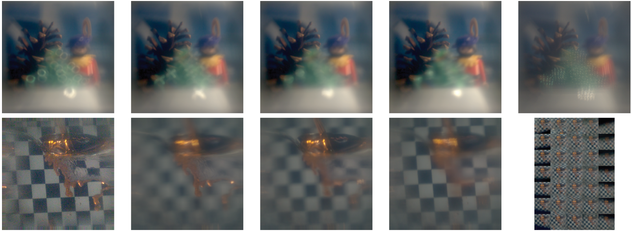
Figure 15: Refocusing results for light fields recorded with a laser cut mirror setup after upsampling to 1617 images (brightness/contrast manually adjusted after recording). The top row shows the result of simulating different aperture shapes for artistic bokeh control, the bottom row demonstrates refocusing for a short-exposure recording of liquid splashing off a spoon. The rightmost column shows refocusing using only the original 35 views (top) and the rectified input views (bottom). Please refer to the supplemental video for more examples.
