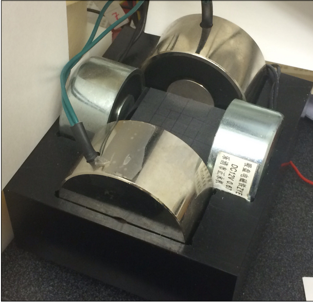
Fig. 7. Our magnetic setup includes 5 electromagnets in a custom-milled holder. Two pairs achieve a relatively uniform field in the x and y axes, while only a single z magnet below the sample (not shown) is used to leave one side open for the projector.
