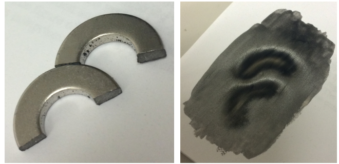
Fig. 6. A spatially varying magnetic field can be used to create spatially varying reflectance. Left : Horseshoe-shaped magnets were placed 3 mm below a sheet of paper. Right : A coating of nail polish was applied to the paper, giving the impression of a bump map. We remind the reader that this sample is completely flat.
