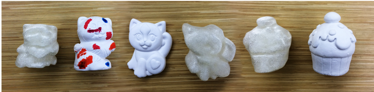
Fig. 12: 3D Printing. We 3D printed the standing cat, flat cat, and cupcake examples. The printed examples showcase the potential of one capture from a passive camera system. Note: we scaled the figurines to fit in a 50mm cube with 0.2mm precision.
