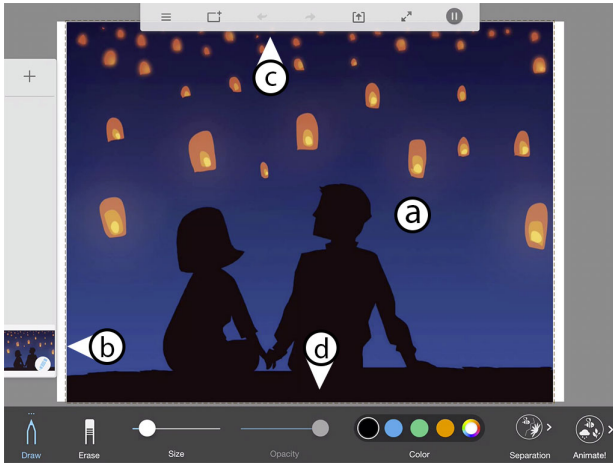
Figure 3: The user interface, consisting of (a) a main canvas, (b) layer panel, the (c) global and (d) contextual toolbars.
