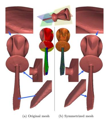
**Fig. 7.** Symmetrizing a scanned screwdriver model. The input mesh is shown on the left side, and the output mesh is on the right. Note that the output mesh is perfectly symmetric, has less noise (e.g., on the tip and at the junction with the handle), and retains sharp features (e.g., the ridge on the top of the handle).
