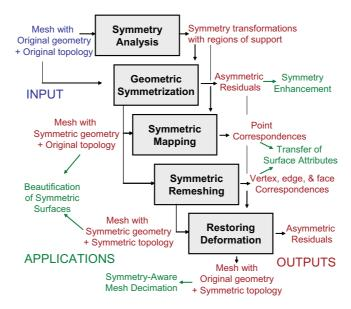
Fig. 1. Symmetry-aware mesh processing framework.
