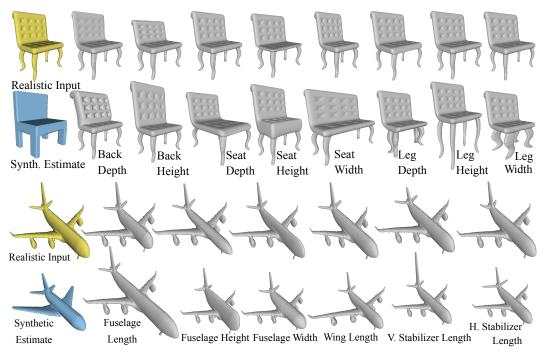
**Figure 4: Editing results with piecewise anisotropic scaling.** Realistic input shapes (yellow) are fit to synthetic templates (blue), then edited by decreasing (top row) and increasing (bottom row) each shape parameter in turn. The proposed method provides for both detail preservation and independent control over each semantic parameter.
