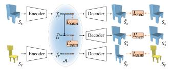
**Figure 3: Learning framework.** We learn a semantic space  $\mathcal{A}$  (blue) by jointly training on synthetic and realistic shapes. Synthetic shapes are supervised in both semantic and shape space, with one reconstruction branch (top) and one editing prediction (middle). Realistic shapes (bottom) are supervised in shape space only.
