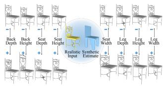
**Figure 1: Semantic editing.** Taking a realistic shape (yellow) as input, the proposed method allows for editing of different parts (gray). This is achieved by learning to infer the semantic parameters of an auxiliary synthetic shape (blue), without any labels from realistic shapes.
