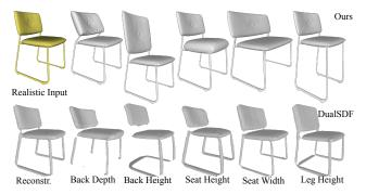
**Figure 8:** Comparison to DualSDF [6]. The input (yellow) is edited by changing a semantic parameter in our system, or adjusting the radius of a primitive in DualSDF. When changing a local parameter with DualSDF, the global shape is also affected, as seen in the alteration or omission of the bottom crossbars on the legs. In addition, in contrast to the proposed method, the DualSDF results lack details such as the button on the chair back.
