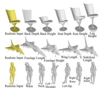
**Figure 6: Editing results for out-of-distribution shapes.** Our method produces reasonable results, and correctly preserves detail, even if the input shape has missing parts or different topology relative to the synthetic template.
