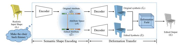
**Figure 2: Framework overview**. To achieve shape editing, we propose a framework that (a) learns a semantic parameter space for both realistic shapes  $S_r$  and auxiliary synthetic shapes  $S_s$  (Sec. 4.1) and (b) transfers the deformation of synthetic shapes to realistic shapes (Sec. 4.2).
