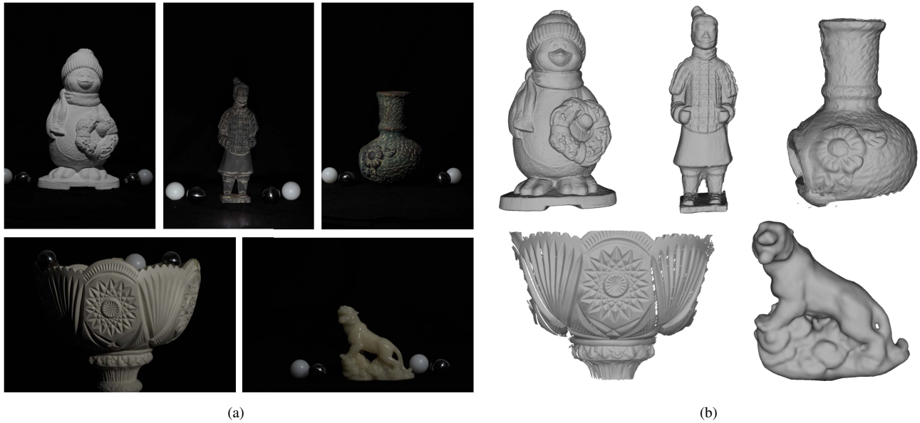
Figure 3: (a) Real-world objects captured under varying illumination with calibration spheres included in the scene, (b) 3D scanned models of the real-world objects on the left.
