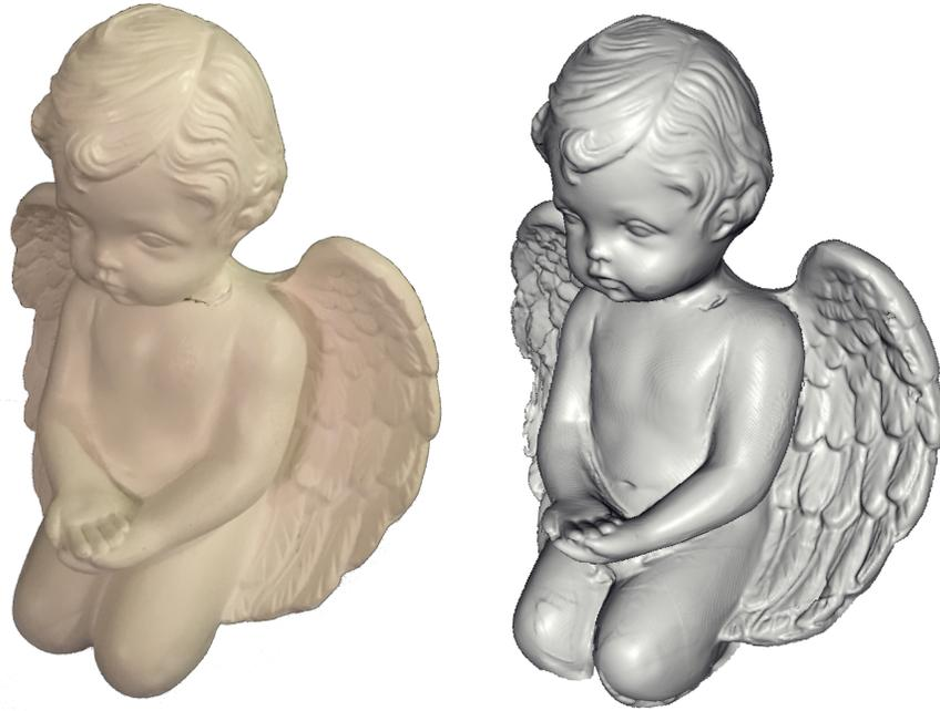
Figure 5.7: A 20 cm tall angel figurine (left) is scanned and reconstructed (right) using our system, with the object platform adjusted to three heights.
