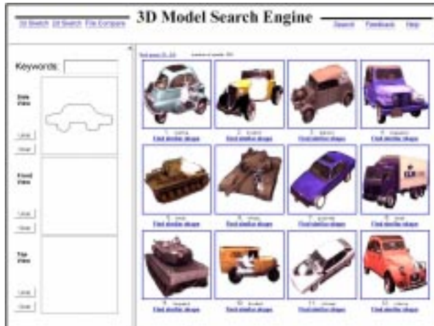
Figure 1: Screenshot of our search engine for 3D models. It allows a user to specify a query using any combination of keywords and sketches (left). Then, for each query, it returns a ranked set of thumbnail images representing the 16 best matching 3D models (right). The user may retrieve any of the 3D models by clicking on its thumbnail, and/or he may refine the search by editing the original input or by clicking on the “Find Similar Shape” link below any thumbnail.
