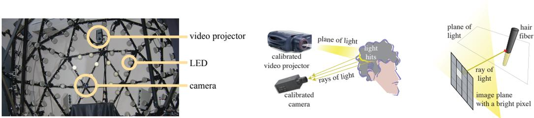
Figure 2.2: Scanning hair strands by Hair Photobooth [58]. The hair strands are triangulated by intersecting the projected plane of light and the rays of light from the camera. Figure reproduced from [58].
