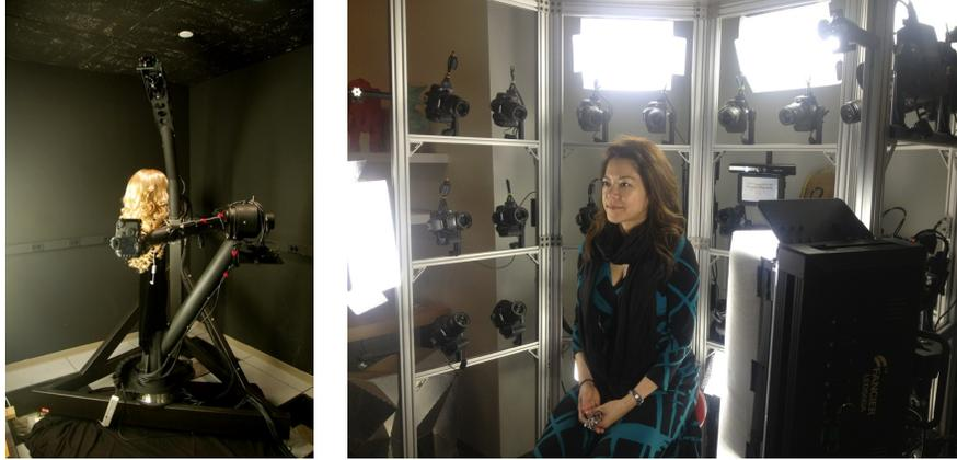
Figure 5.12: We use a robotic gantry to position an SLR camera at 50 views to capture the images for the wigs (left). For real hairstyles, we use a camera array of 30 SLR cameras (right).
