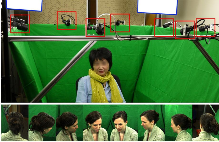
Figure 4.2: Our hair capture setup and a few sample images. We use 8 cameras (outlined in red) in wide-baseline to capture the complete hair styles. Four area lamps (outlined in blue) are used to compensate for the short exposure time.
