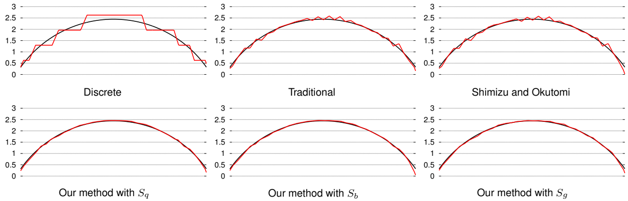
Figure 9: Depth profiles for a synthetic spherical model (5mm radius). For each plot, ground truth is shown in black. Note the reduced noise level for a variety of matching ridge slopes (produced by the varying object tangent).
