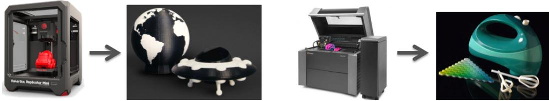
Figure 1.1: Current 3D printing systems are limited in the richness of material appearance they can reproduce. Cheap printers, like the Makerbot on the left, can only fabricate two colors and even expensive printers, like this Objet Connex on the right, can achieve full color but are limited in the materials it can use.
