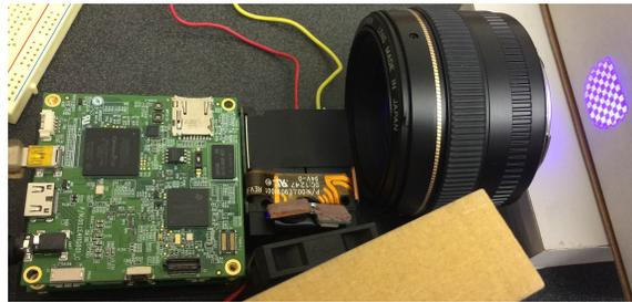
Figure 3.11: We used a lens in reverse to focus the light. This resulted in a small image but large enough given our target area of only 1x1cm.
