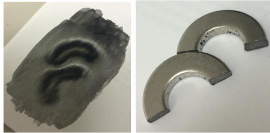
Figure 3.6: A spatially varying magnetic field can be used to create spatially varying reflectance. A coating of nail polish was applied on paper while the two magnets on the right were placed 3mm below the paper. The resulting flake orientations gives the impression of a bump map. We remind the reader that this print is completely flat.
