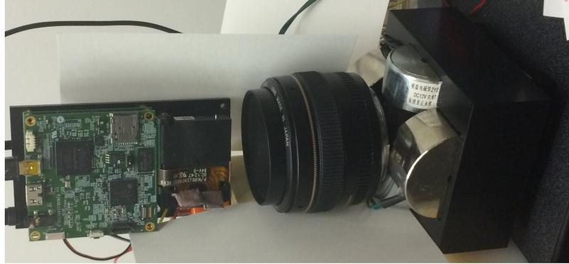
Figure 3.10: We use a projector powered by a UV-led to selectively harden individual pixels. For BRDF fabrication, we apply a magnetic field (or a field schedule) and then harden all pixels compatible with the applied field. We then switch the field and harden other pixels. Printing proceeds in multiple passes.
