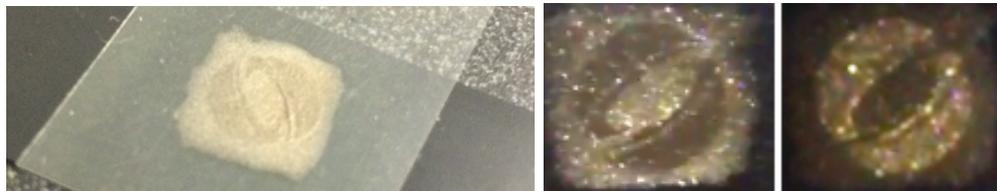
Figure 3.25: Siggraph logo where foreground and background have different anisotropic tangents. This print was created using the spiral field to randomize the flakes orientations followed by the line field to achieve the anisotropic distribution. This process was repeated for foreground and background. On the left, lit under a natural environment. On the middle and right: lit with a point light from different azimuthal angles at constant elevation.
