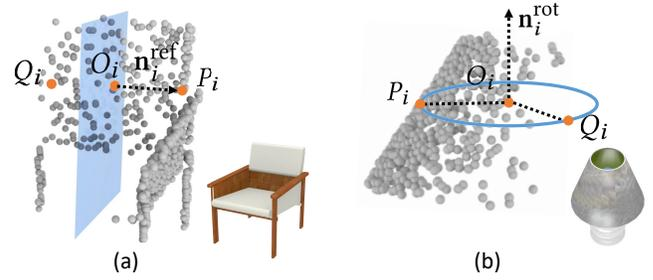
Fig. 3. Demonstration of the relationship between the to-be-predicted point  $P_i$ , its counterpart  $Q_i$ , and  $O_i$  which is the projection of  $P_i$  onto (a) the predicted symmetry plane with the plane normal  $\mathbf{n}_i^{\text{ref}}$  for reflectional symmetry and (b) the predicted symmetry axis with the unit vector  $\mathbf{n}_i^{\text{rot}}$  for rotational symmetry.
