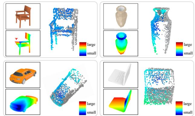
Fig. 12. Visualization of the predicted counterparts. The grey points represent the input points. The colored points are the predicted counterparts, where the color encodes the Euclidean distance between the location of the predicted counterparts and their ground-truth location (i.e. the Euclidean distance error). Referring to the color bar, the warmer the color, the larger the error is.
