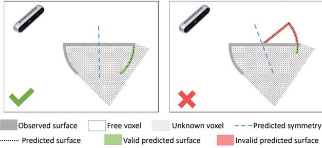
Fig. 5. Verification of the symmetry prediction based on the matching error which is equivalent to the overlap between the transformed points  $T(P)$  and the regions of space that are known to be free.
