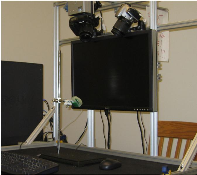
Figure 5.5: Photograph of our experimental setup. The object is placed in front of the monitor, facing the camera pair. The cameras capture image pairs while the monitor displays sweeping linear light sources. The small projector visible above the cameras is used for comparison with structured-light reconstructions.
